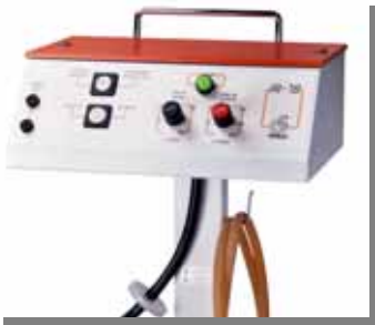
Panel de mandos con selector de continuos intermitentes Control panel with continuous or intermittent selector
